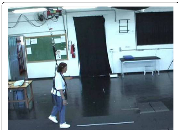
Figure 1 Partial view of a gait training session with the body weight support system used in the study. The rail that the electric motor slides along, the load cell, and one of the participants of the study wearing the harness are shown.
